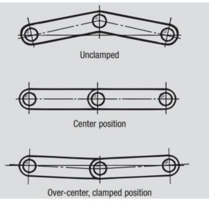
Toggle action clamps operate through a linkage system of levers and pivots. The fixed-length levers, connected by pivot pins, supply the action and clamping force.
